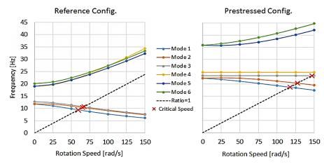
Figure 4. Campbell diagram for reference and prestressed configurations
